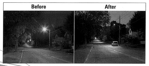
LEDs have better, broad spectrum lighting than traditional high pressure sodium cobra head-style streetlights which spill excessive yellowish-orange light away from the street and into neighboring yards and windows. Because existing poles are not being moved, any unlit areas between poles (corners and midblock locations) are unchanged. However, due to the uniformity of the light from LEDs, the difference between lit and unlit areas is accentuated.
